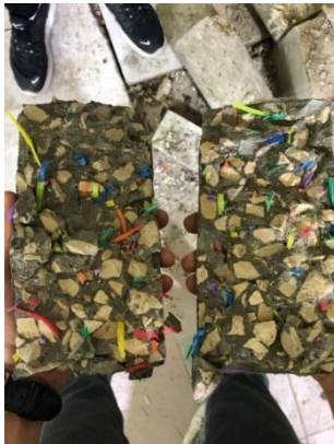
Fig.13. Fiber distribution after testing PS-0.5 sample
