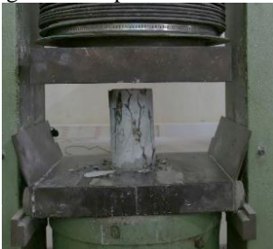
Fig. 6. Sample under compressive strength test
