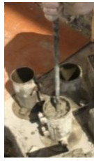
Fig.4. Compacting using a tamping rod
