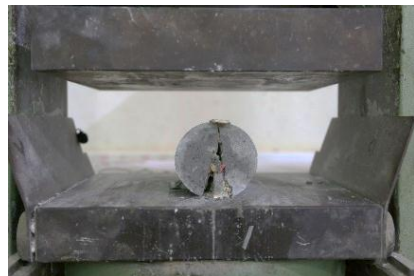
Fig. 7. Sample under splitting tensile test
