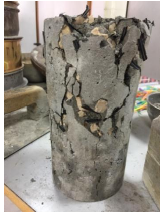
Fig. 11. Damaged cylinder from PS-0 sample
