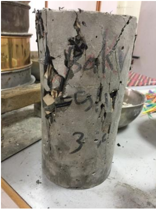
Fig.10. Damaged cylinder from PS-3 sample
