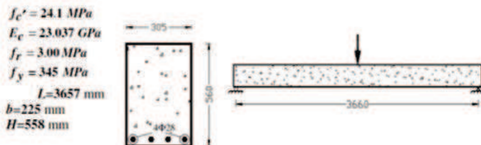
Figure (6): Details of a reinforced concrete simply supported beam under concentrated load at mid span with (L/H=6.55) ( kreshna)
